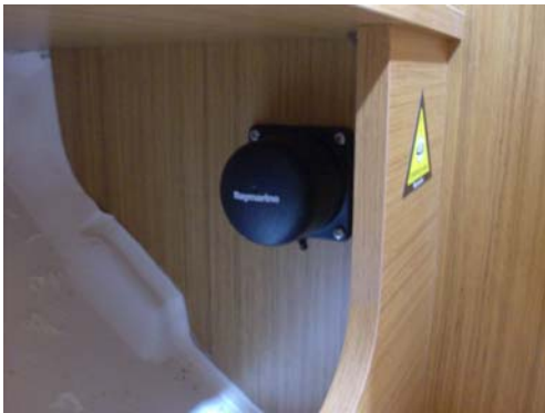
Gyrocompass - Hanging locker - Port aft cabin
