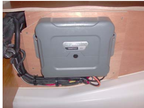
Vessel Management Unit - bulkhead - Starboard aft cabin
