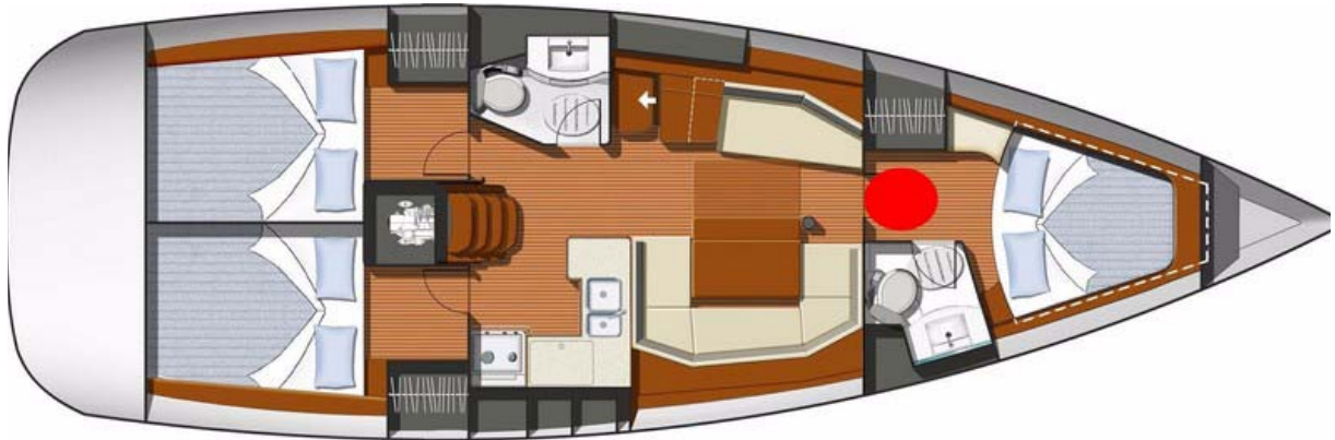
Log and depth sounder transducers View interior
