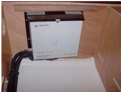
BATTERY CHARGER 12/220V - 40A - Location: Starboard aft cabin
